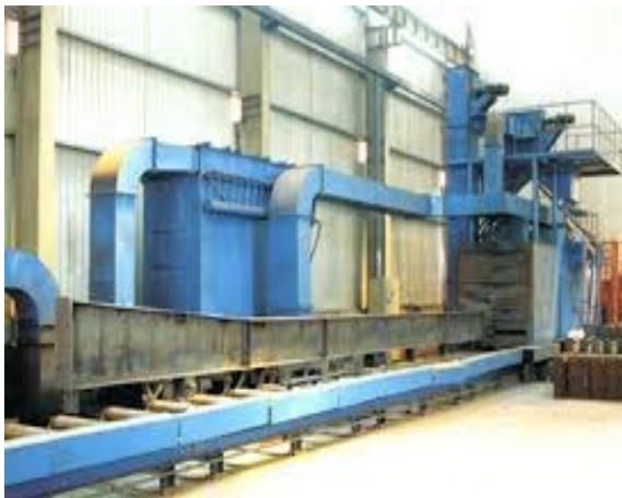
Controlled Atmosphere/Blast Cleaning
