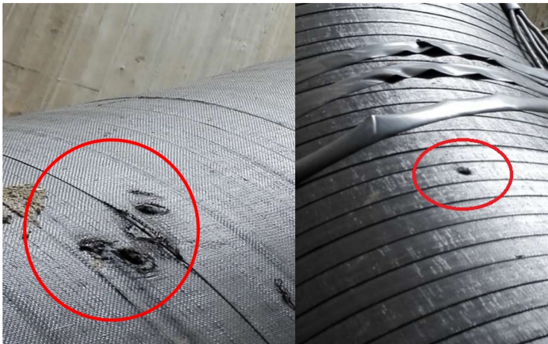
Fig. 2 On-site Collision Damage of the hot-bending bends
