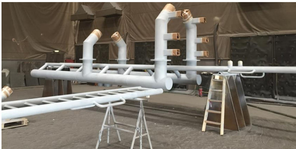
Figure 1: Boatlandings and ladders duplex coated (2)
