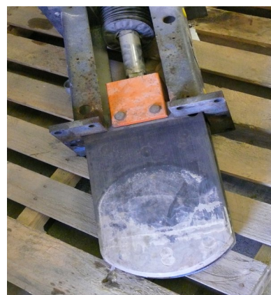
Figure 6: Knife gate no corrosion
