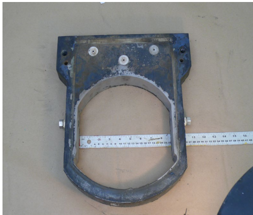
Figure 5: Center valve body no corrosion
