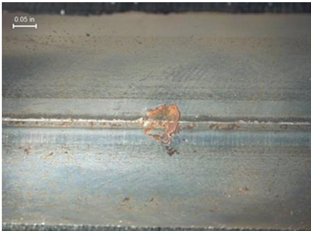
Figure 2: Macro view of visible pitting along the seam weld in an area without any significant deposit present. The location of the tube seam weld and the associated corrosion products (rust) are visible.
