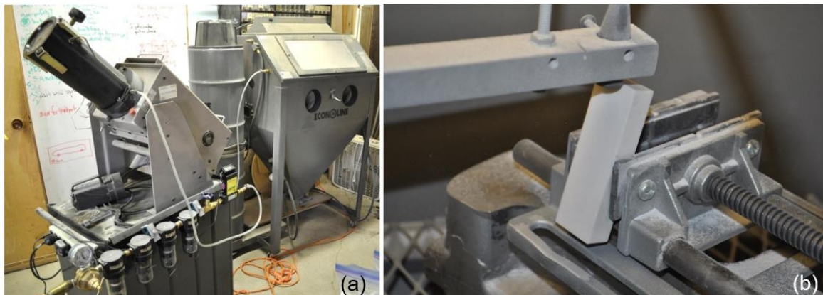
Figure 1: (a) ASTM G76 erosion testing set-up (b) nozzle and sample holder inside containment cabinet
