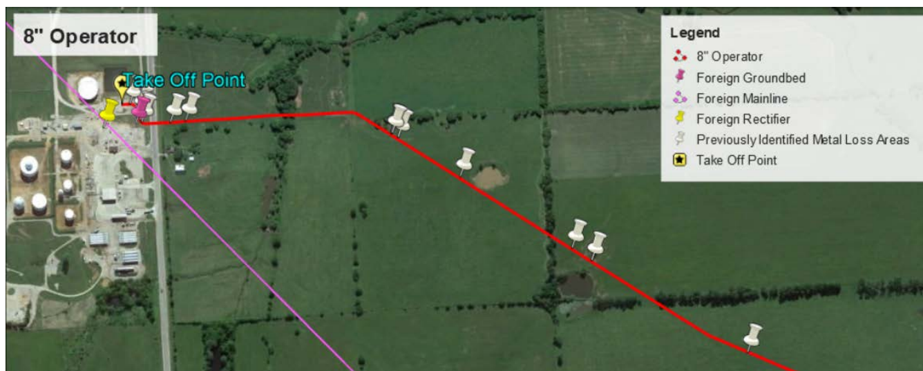
Figure 3: Operator pipeline near take off showing metal loss areas
