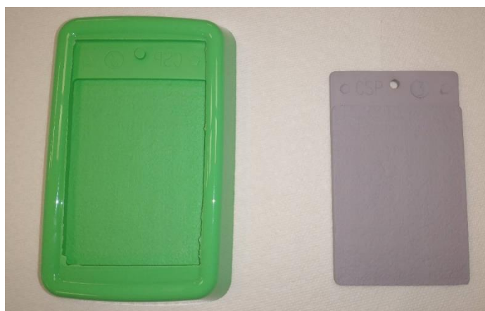
Figure 2: The silicone mold of ICRI CSP Chip 3
