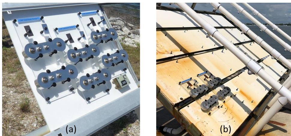
Figure 2: Atmospheric exposure test panel at NRL Key West site (seawater spray rack shown on right)
