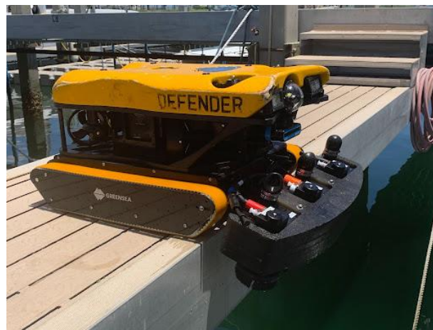
Figure 1 - Crawler and Groomer mounted to VideoRay MSS Defender
