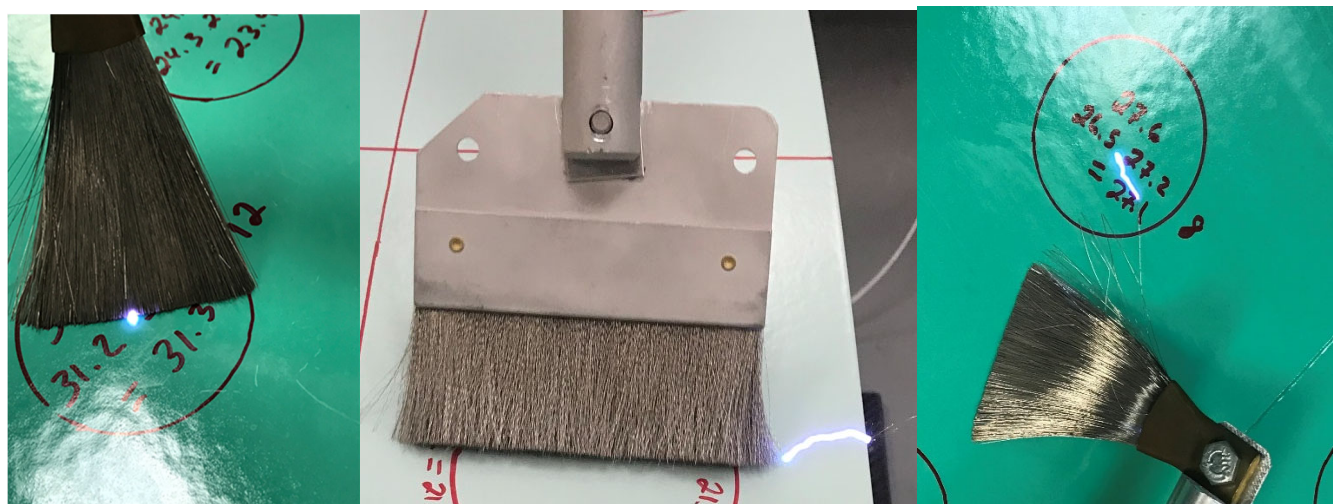
Figure 1: Examples of Voltage Exceeding Dielectric Strength of Air and Generating a Visible Spark
