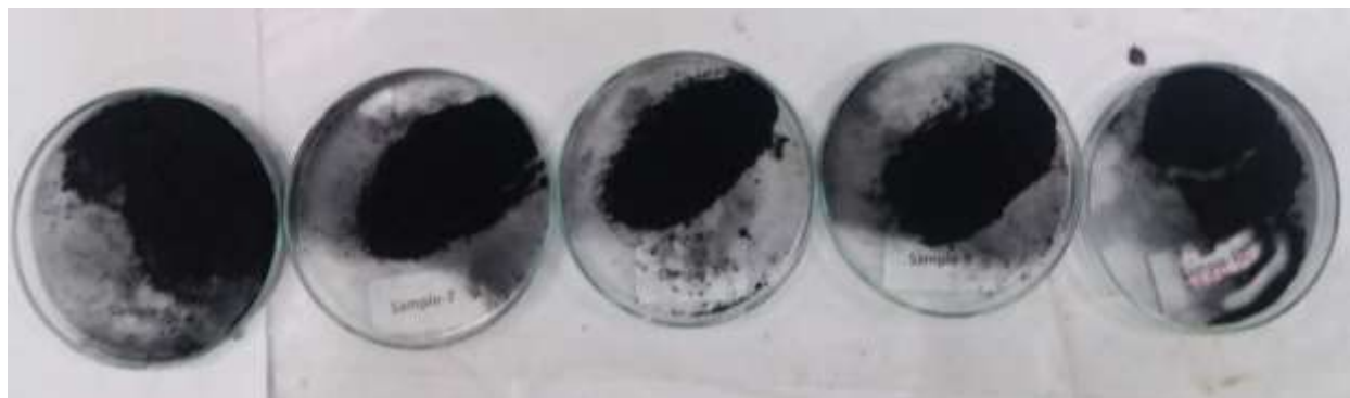
Figure 3: Experiment Samples in Petri Dish for Oxidation of Iron Sulfides (FeS) from Black Powder Deposits
