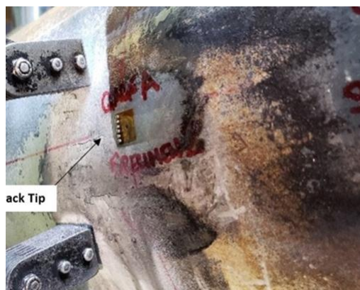
Figure 5: Residual Stress Measurement Locations and Photo of Location A
