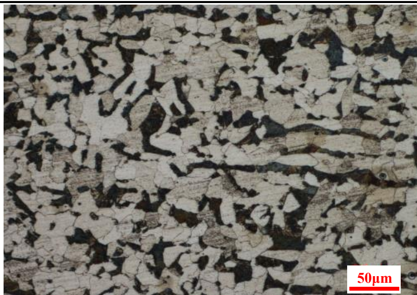
Figure 1: Microstructure of X60 steel
