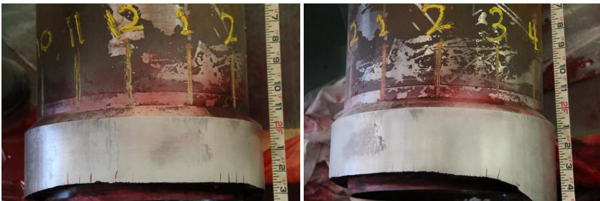
Figure 7: Photographs of the PT examination on the Top Sub external surface.
