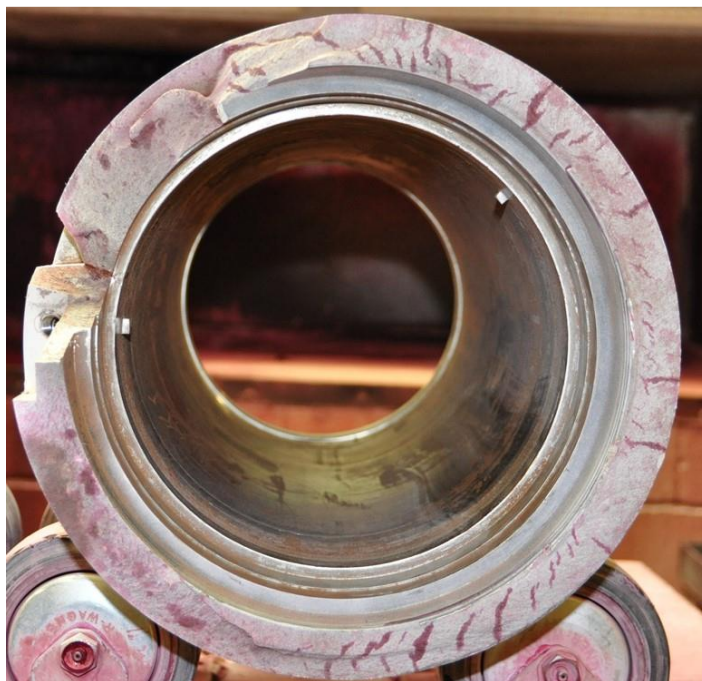
Figure 8: NDE evaluation of long section of fracture Transverse Cross-section showing multiple secondary cracks
