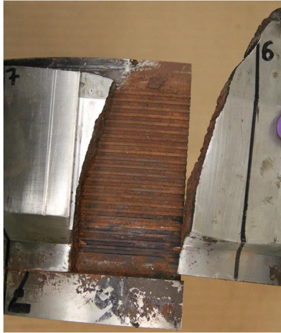
Figure 6: Photograph of the longitudinal control line milled pocket crack after sectioning
