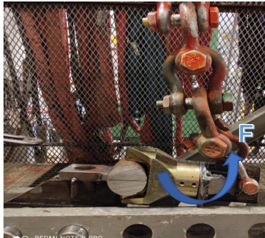
Figure 4: Close-up of Torsion Load Test of Clamp attached to the mooring chain section.
