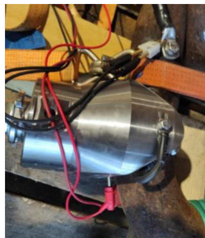
Figure 5: Electrical Continuity Test Setup, Clamp attached to the mooring chain section.
