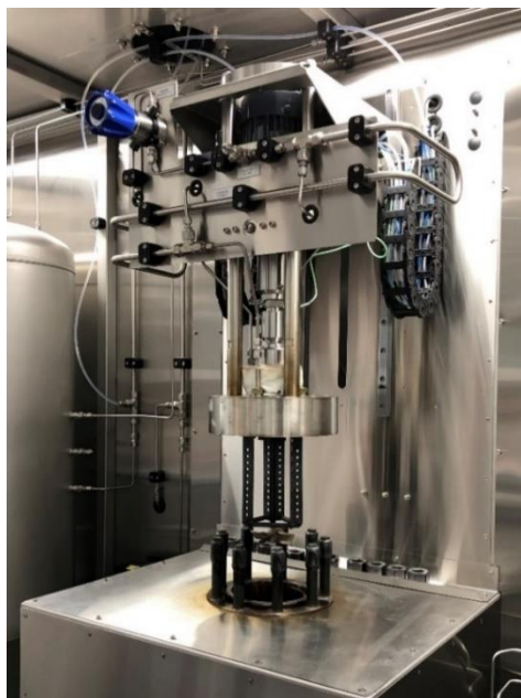
Figure 2: The autoclave with the lid opened before installation of test samples.
