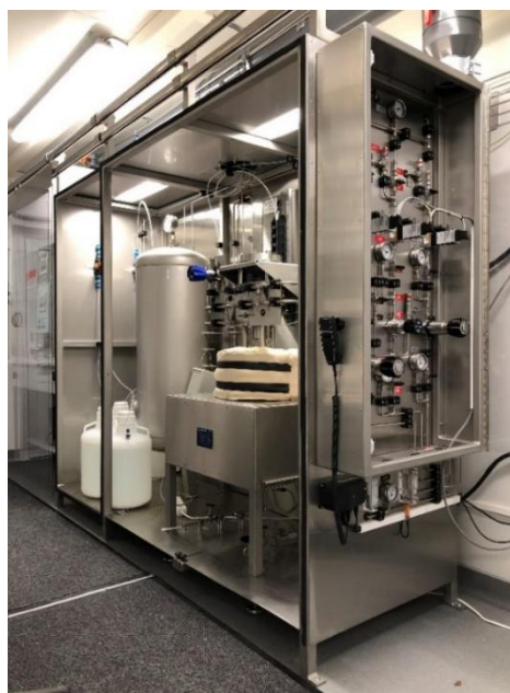
Figure 3: Experimental setup with filling panel (right) and H 2 S capture system (left).
