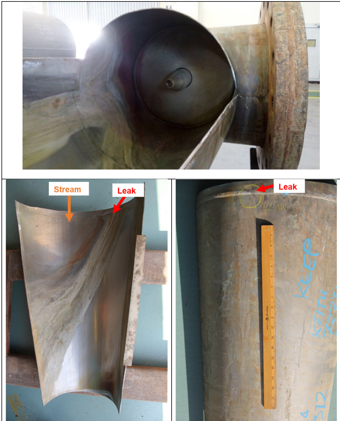
Figure 2: General photographs of the leaked venturi scrubber (ejector) after cutting.
