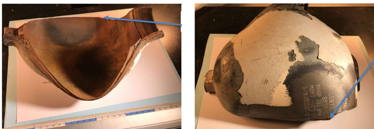
Figure 3: Retrieved part of dampener showing high degree of deformation
