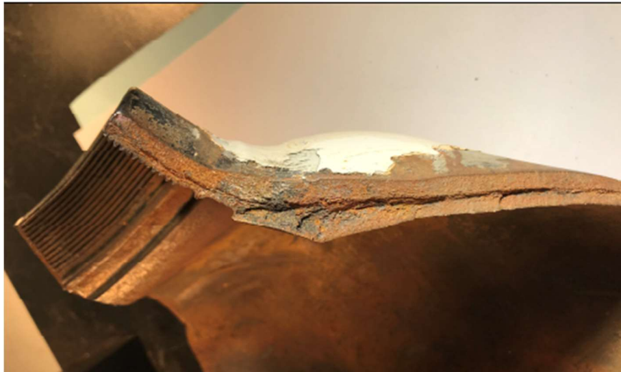
Figure 6: Fracture surface with stepped appearance and curved steps on inner facet
