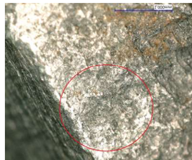
Figure 5: Suspected area of fatigue initiation at component marking area confirmed to be free of typical striations by SEM.
