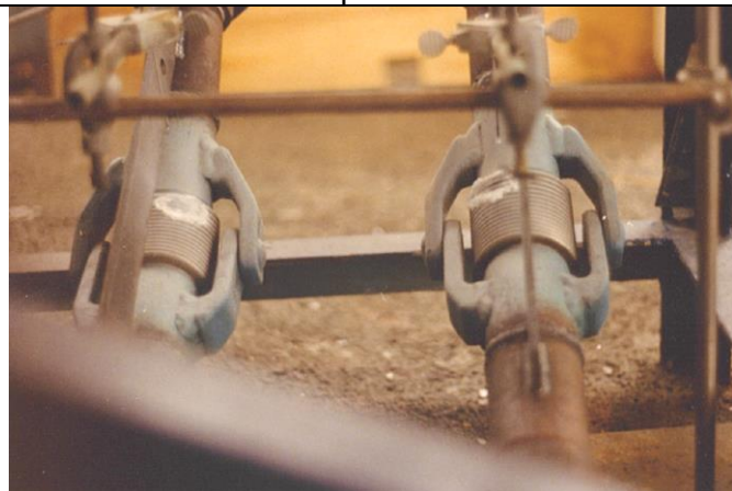
N08825 (left) and S32100 (right) with brine drip.
