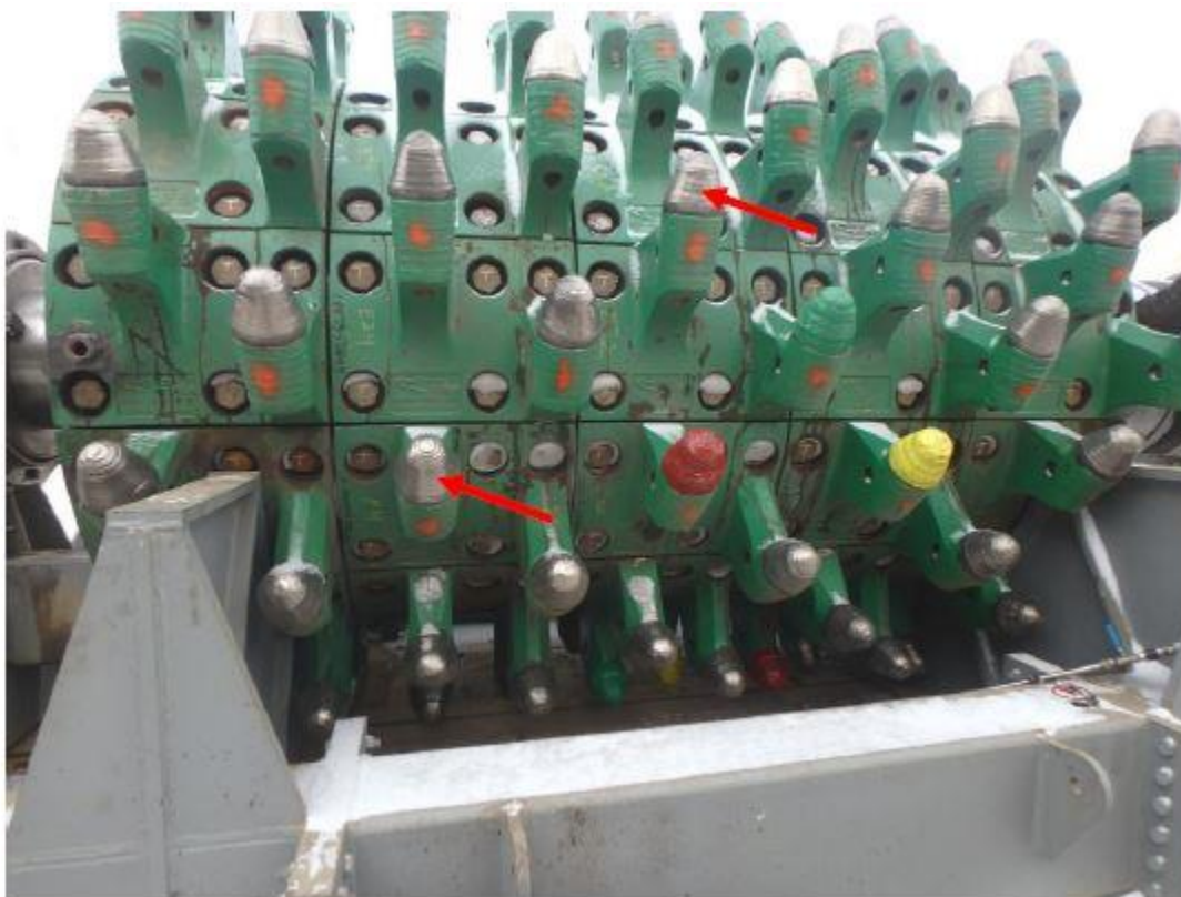
Figure 2. PTAW WCO/carbon steel double-roll crusher teeth.
