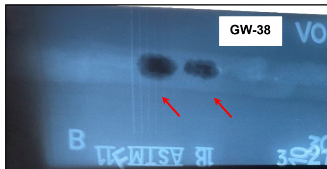
Figure 4. Section of the radiograph showing internal voids for pipe segment GW-38.
