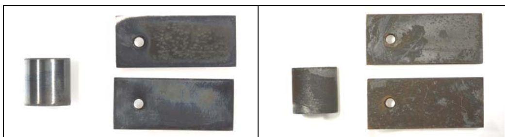
Figure 2. Examples of visibly uneven corrosion in tests with no precorrosion. Inhibitor 1 (left) and Inhibitor 2 (right)
