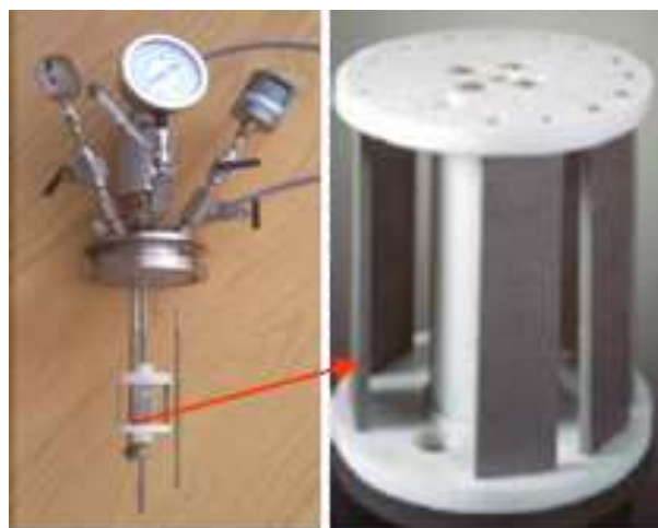
(b) Rotated cage with test coupons
