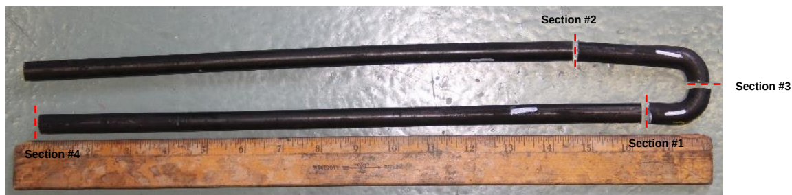
Figure 3: photograph of failed sample (Case 1)
