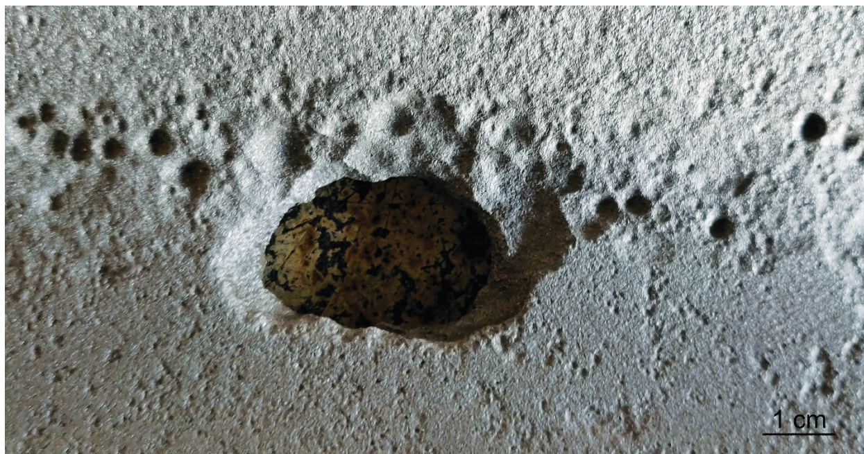
Figure 2: Close-up photograph showing several deep pits surrounding perforation on FL1
