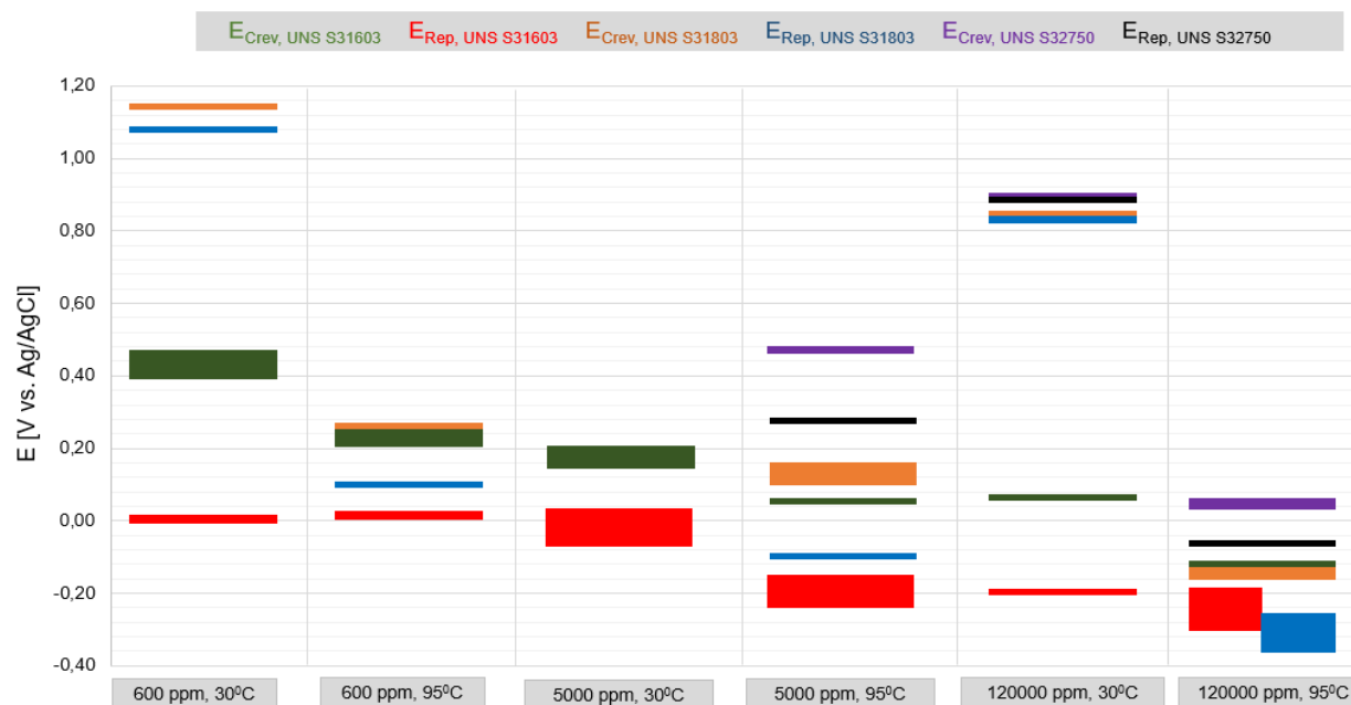
Figure 2: Summary of E_{rep} and E_{crev} measured for different temperatures, Cl^- - ion content and alloys 19 .
