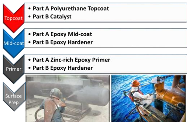
Figure 1 Three-coat system on prepared steel
