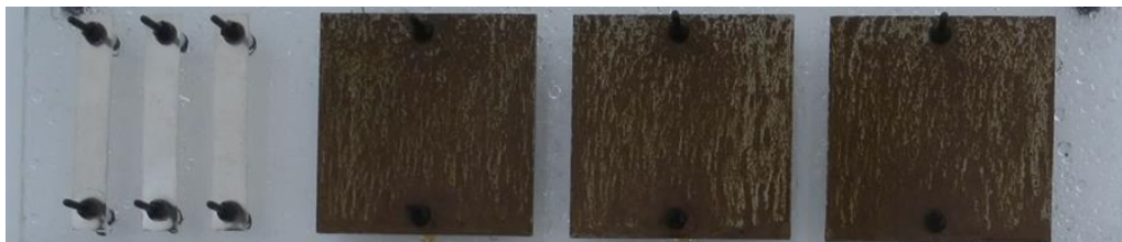
Figure 3: Representative image of the silver and steel coupons deployed in this investigation. These samples are shown after two months of the daily sea water spray with the weekly CWR.
