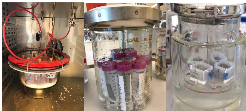
Figure 3: Test setup for \text{SR}_{\text{FeCO}_3} experiments. Wires are exposed in small containers mounted in large test cells. The test cells are continuously gas flushed. Water samples are taken with a syringe through holes in the lids.
