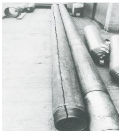
Figure 1: Cracking in the 22% Cr DSS Cold Worked Tubulars 7
