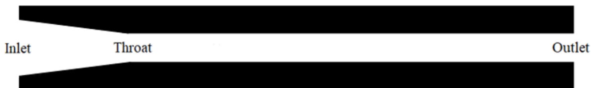
Figure 2. Straight bore nozzle geometry
