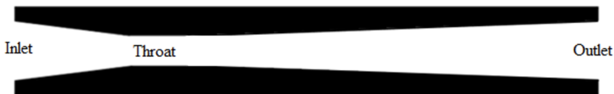
Figure 3. Venturi nozzle geometry
