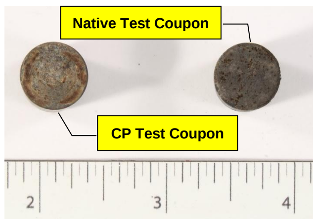
Figure 12: Photograph showing cut sections of the CP & native test coupons from the test station after ultrasonic cleaning.
