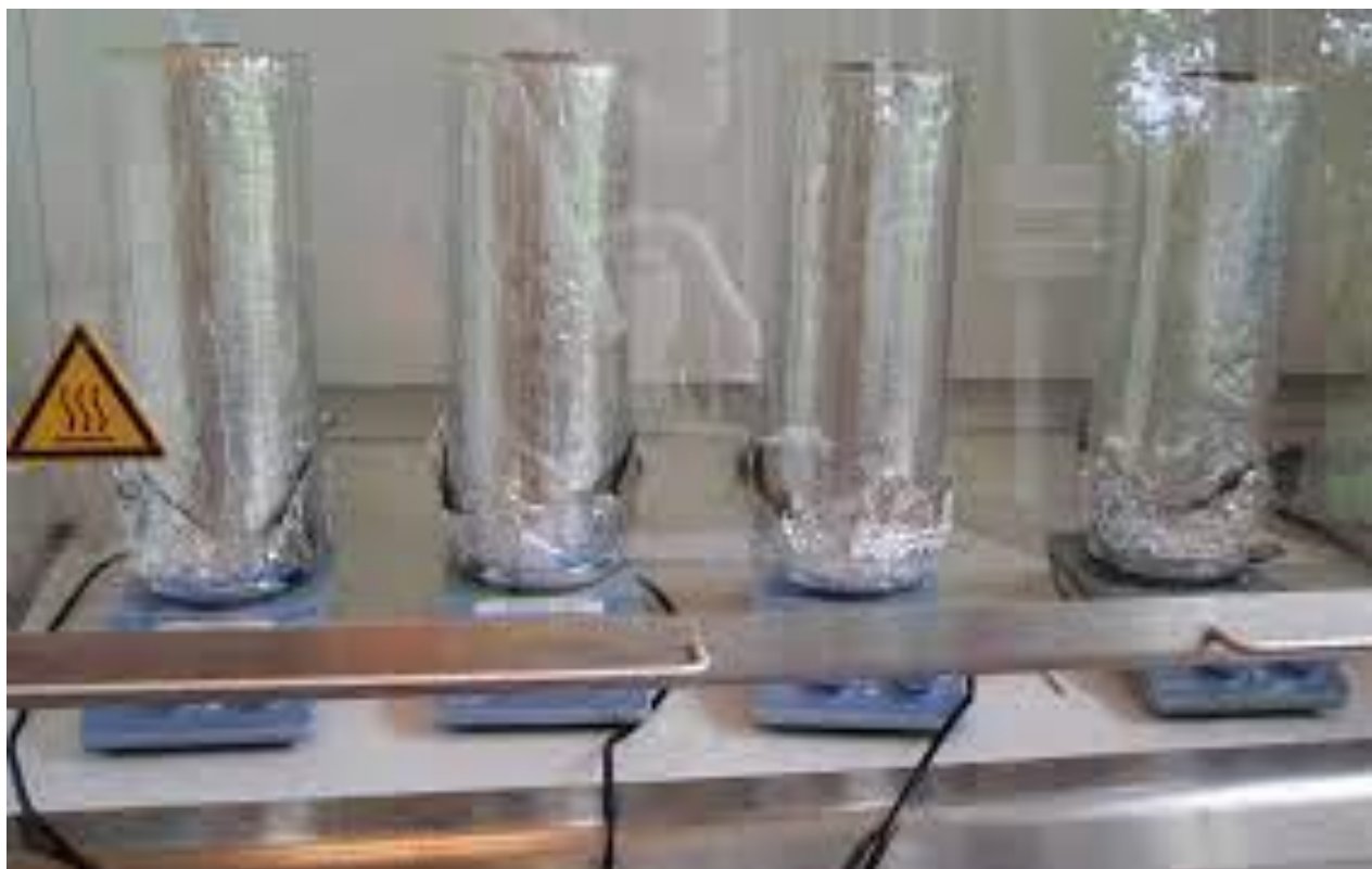
Figure 2: Houston pipe test showing insulated pipe sections on hotplates
