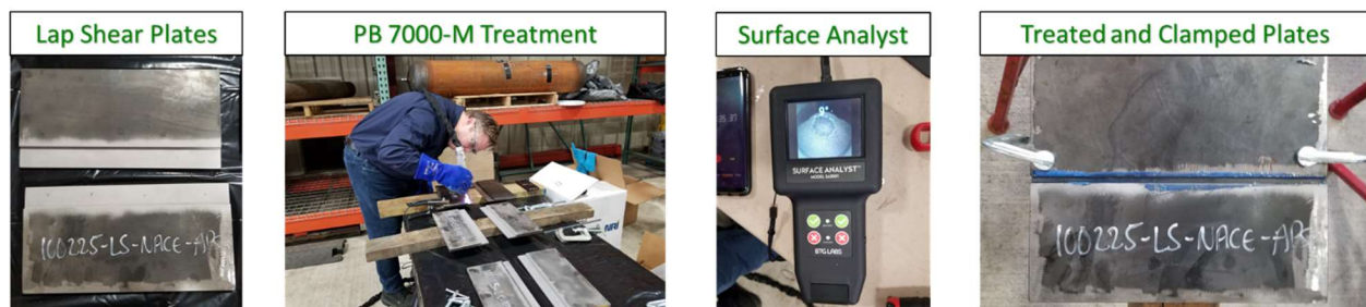
Figure Error! No text of specified style in document.: Lap Shear Samples Surface Preparation and Assembly
