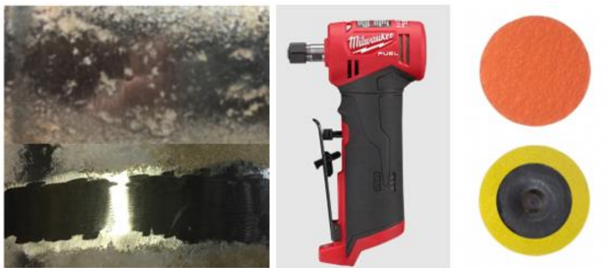
Figure 5. Prepared pipe sample with surface pitting removed using ceramic disc
