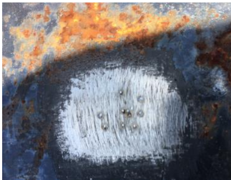
Figure 4. Measurements effects of poor sample preparation
