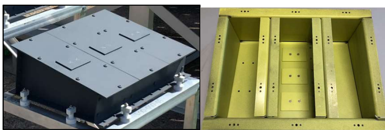
Figure 1: Photographs of the simulated aircraft structures (SAS) used for sensor exposures
