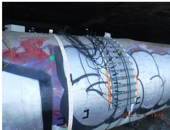
Photo 2. BEM scanning of cement mortar coated steel pipe.
