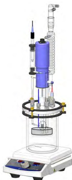
Figure 5. Overview of the RCE experimental setup and test matrix.
