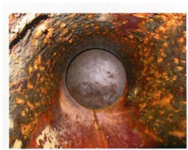
Figure 2: Corroded Carbon Steel Discharge Pipe – Before Cleaning
