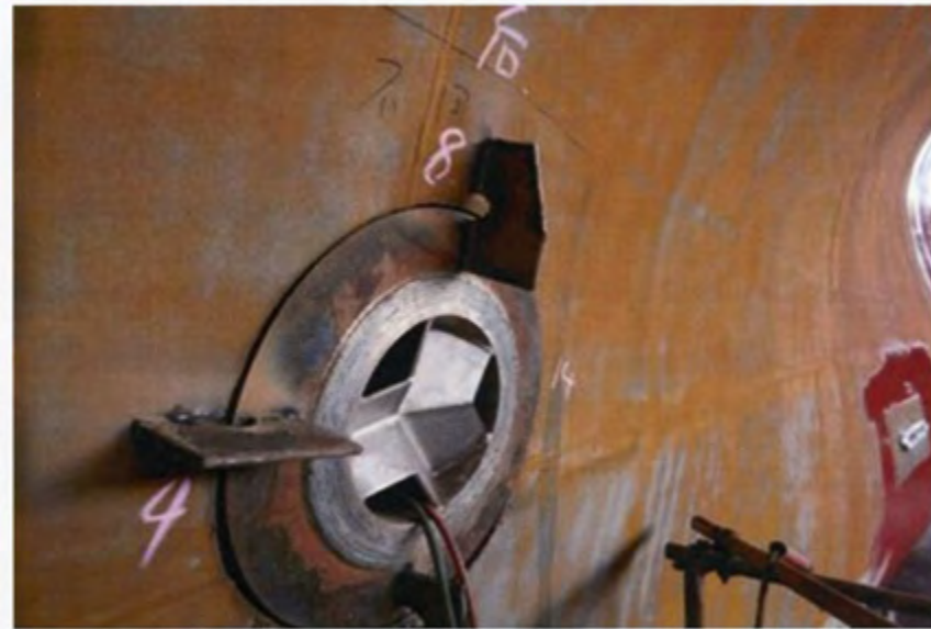
Figure 5: Discharge Stub Pipe Exiting Hull with UNS (1) S31254 Pipe Welded with Alloy 625, and Alloy 625 Weld Overlay (Cladding) around the Washwater Discharge Outlet
