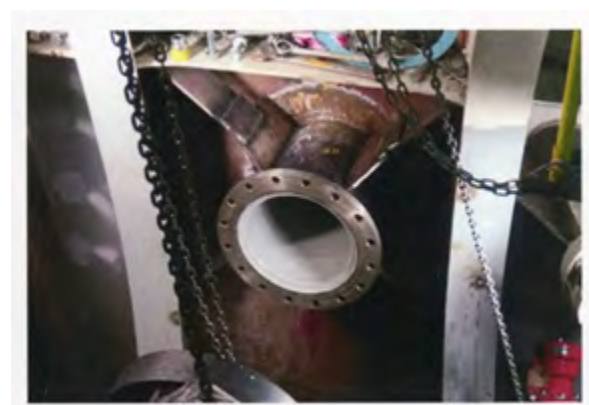
Figure 4: A New Discharge Stub Pipe Installed in a Ship Ready for Service
