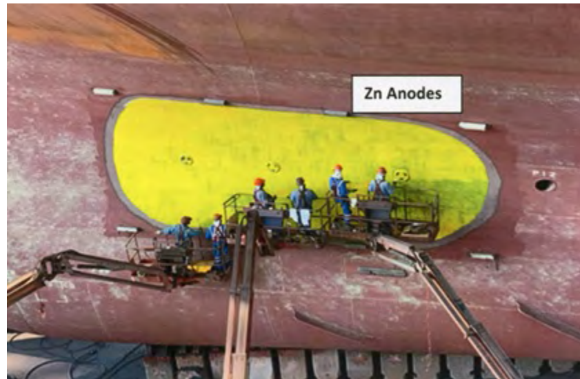
Figure 6: Discharge Stub Pipe Exiting Hull with Marine Coating System and CP System (Zinc Anodes)
