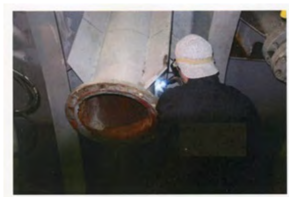
Figure 3: Removal of a Corroded Discharge Stub Pipe from the Hull of a Ship
