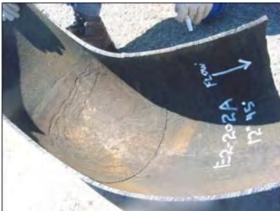
Figure 3-2-4—Preferential corrosion in an amine regenerator reboiler return elbow. (Reference 6)
