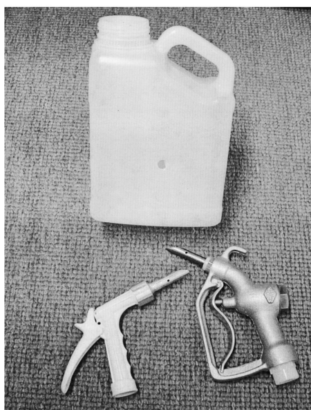
Figure 2 – Examples of pressure nozzles and a punctured container
