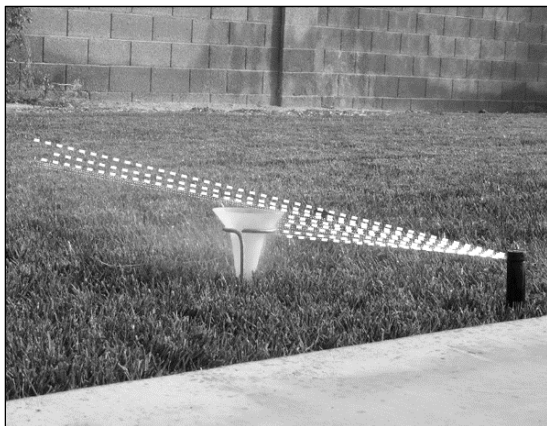
Figure 4 – Incorrect placement of catch device
