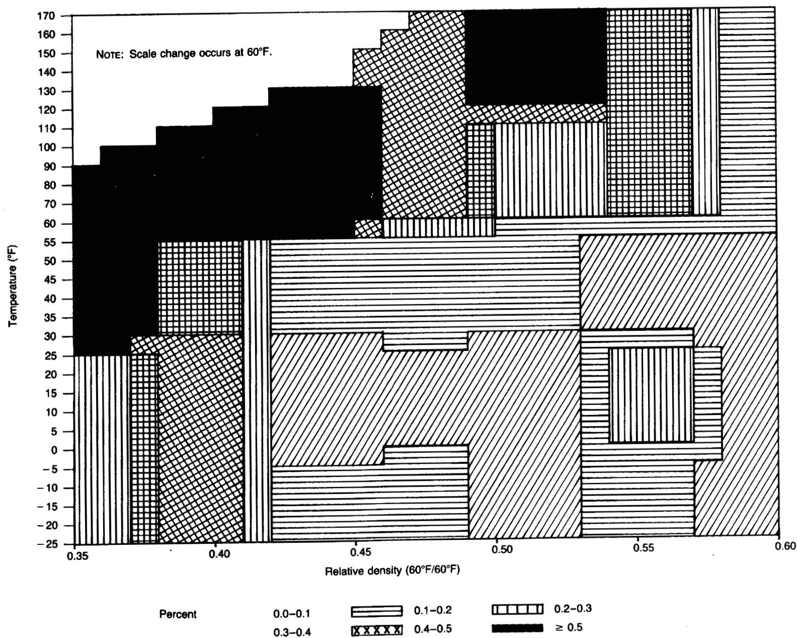
Figure 2—Uncertainties (95-Percent Confidence Level) in Volume Versus Temperature and Relative Density
