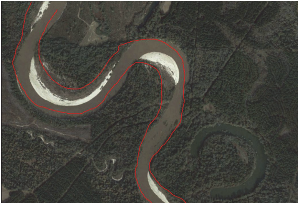
Figure 5—2013 Aerial Photograph of the Leaf River, MS Illustrating Significant Bank Erosion and Channel Migration. Note: Red line indicates approximate location of river banks in 1996
