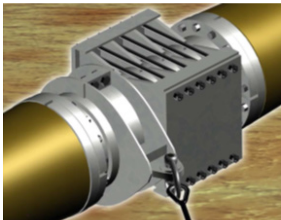
Figure 25—Close-up View of Tether Clamp
