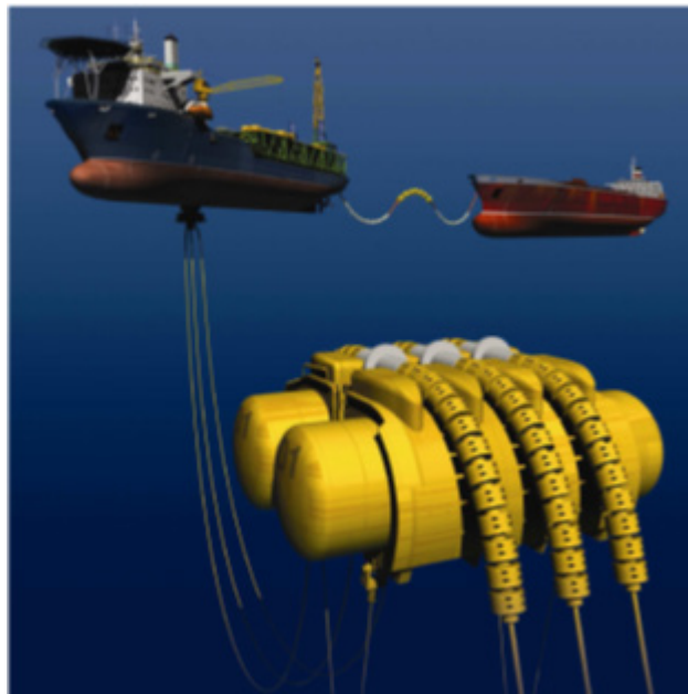
Figure 20—Subsea Buoy with Buoyancy Tanks, Showing Gutters
