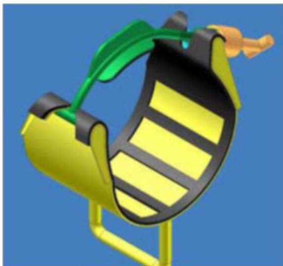
Figure 29—Light-weight Repair Clamp [35]
