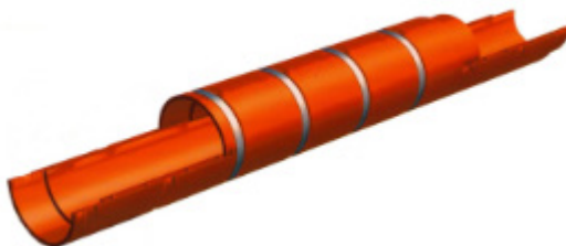
Figure 44—Example of Flexible Pipe Abrasion and Impact Protection
