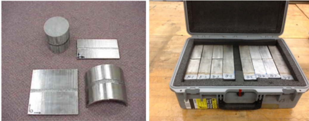
Figure 1—Photograph of Performance Demonstration Test Sets for Detection and Characterization (left) and Crack Sizing (right)
