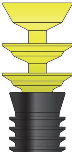
Figure 3—Example of Combination Cementing Wiper Plugs
