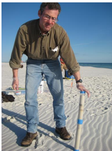
Figure 8: Core sample in a transparent sleeve obtained from the supra-tidal zone (i.e., landward of the high water mark). The discoloration at approximately one third from the top represents oil deposition.
