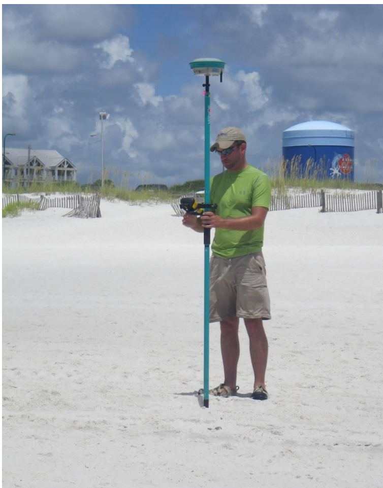
Figure 4.1 GPS Satellite Survey Equipment
